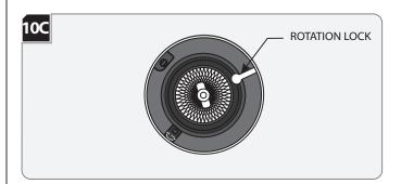
**NOTE:** Lamp housing can rotate 361° horizontally.
